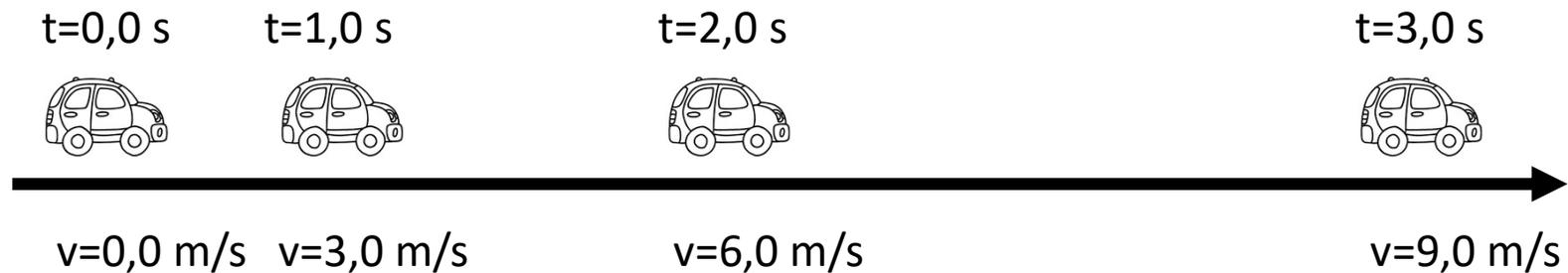
$$a = \frac{\Delta v}{\Delta t} = \frac{3,0 - 0,0}{1,0} = \dots = \frac{9,0 - 6,0}{1,0} = 3,0 \frac{m}{s^2}$$
